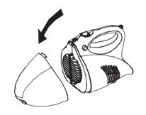
Pull out the dust bag/filter, by grasping the side of the filter and pulling out.
