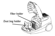
When vacuuming fine dust particles, the fine dust particles can clog the pores of the dust bag and the dust bag indicator will indicate full. If this happens the bag could appear relatively empty, however the bag will still need to be emptied to avoid strain on the motor. NOTE: The bag compartment lid may not close if the bag is not correctly fitted.
