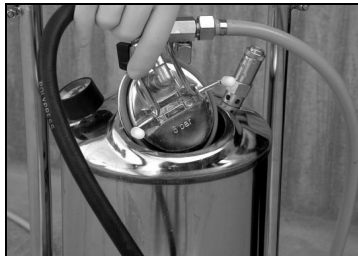
Insert cap in pressure vessel opening
