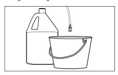
**Step 3** Fill a container with Karcher detergent. Place the filter end of detergent suction tube into the container.
