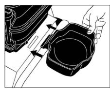
**Step 4** Insert the detergent tray into the tray slot and screw in the fastener. Fill the detergent container with the proper detergent for you cleaning project. Note: Place the container on the trav.
