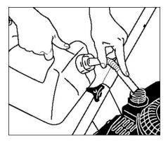
**Step 5** Fill gas tank with unleaded gasoline. Do not use leaded gasoline.
