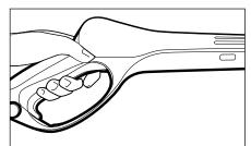
**Step 4** With the engine running, pull trigger to operate unit: Liquid detergent is drawn into the unit and mixed with water. Apply detergent to work area. Do not allow detergent to dry on surface.
