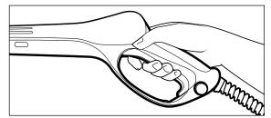
**Step 4** Trigger the gun to eliminate trapped air, wait for a steady flow of water to emerge from the spray nozzle.
