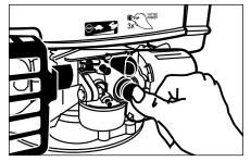
**Step 6** Push primer ball three times. Wait 3 seconds between each push. Note: in cold weather push 5 times.
