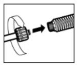
Step 3 Attach the wand to the spray gun.
