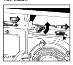
Step 5 (Briggs & Stratton) Turn fuel valve to "ON". Slide the throttle control to the fast position. Move the choke lever to the "CHOKE" position (only if the engine is cool). After starting, move the choke to "RUN".
