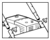
Step 1 Attach the handle to the frame of the pressure washer. Align holes, insert bolts, and tighten with knobs.
