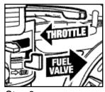
Step 6 Slide or turn the fuel valve to the on position. Slide the throttle lever toward the fast position.
