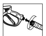
Step 7 Attach the high pressure hose to the spray gun.
