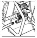
Step 6 Disconnect garden hose from water inlet on the unit.
