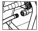
Step 9 Connect the garden hose to unit's water inlet.
