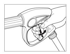
**Step 5**Trigger the gun to eliminate trapped air, wait for a steady flow of water to emerge from the spray nozzle.
