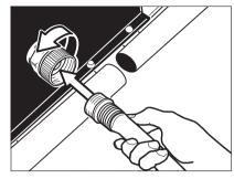
**Step 2** Connect water supply hose to unit's water inlet.
