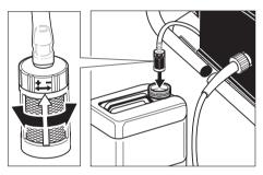
**Step 2**Adjust the filter end of the detergent tube for light (-), or maximum (+) detergent coverage. Place the filter end of detergent suction tube into the jug.
