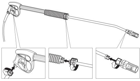
**Step 1**Attach the high pressure hose to the spray gun.
