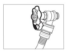
**Step 3**Connect water supply hose to the cold water source and turn water on completely.
