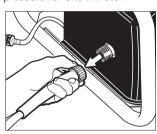
**Step 5** Disconnect the garden hose from the water inlet on the unit.
