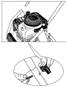
Step 2 Align the holes of the accessory rack to the handle and fasten the four screws.
