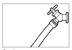
Step 5 Connect garden hose to the cold water source and turn water on completely.
