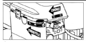
Step 7 Slide the throttle control to the fast position. Move the ckoke lever to the "CHOKE" position (only if the engine is cool). After starting, move the choke to "RUN".
