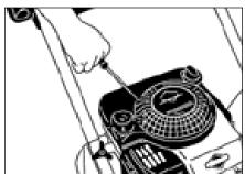
**Step 6** Pull the starter handle. If the engine fails to start after 3 pulls squeeze the trigger gun to release pressure, and repeat step 7.
