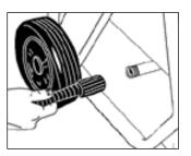
Step 6 Disconnect the high pressure hose from the high pressure outlet and engage the gun safety lock.
