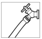
Step 3 Connect garden hose to the cold water source and turn water on completely.
