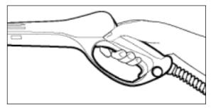
**Step 4** Trigger the gun to eliminate trapped air, wait for a steady flow of water to emerge from the spray nozzle.
