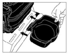
Step 4 Insert the detergent tray into one of the slots of your choice and screw in the fastener. Fill with the proper detergent for your cleaning project. Place the container on the tray.
