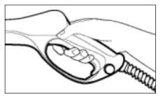
Step 4 With the engine running, pull trigger to operate unit: Liquid detergent is drawn into the unit and mixed with water. Apply detergent to work area. Do not allow detergent to dry on surface.
