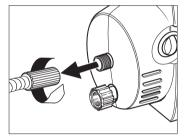
**Step 6**Disconnect the high pressure hose from the high pressure outlet and engage the gun safety lock.
