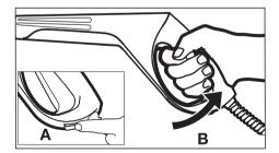
**Step 5**Plug the power cord into the power outlet.
