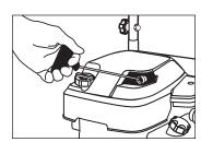
**Step 8** Pull the starter handle. If the engine fails to start after 3 pulls squeeze the trigger gun to release pressure, and repeat step 8.
