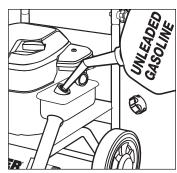
**Step 4** Fill gas tank with unleaded gasoline. Do not use leaded gasoline.
