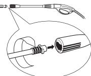
**Step 2** Insert the spray wand into the wand extension. Push in and turn clockwise to lock spray wand in place.
