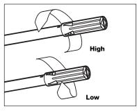
Turn the wand nozzle clockwise to high, for pressure cleaning. Turn counter clockwise to low, to apply detergent.
