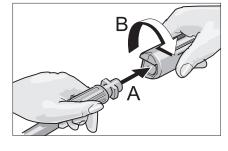
**Step 2**Insert the spray wand of your choice into the trigger gun. Press in against the spring tension (A) and twist into the locked position (B).
