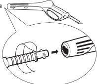
**Step 2** Insert the Vario spray wand into the gun. Push in and turn clock-wise to lock spray wand in place.
