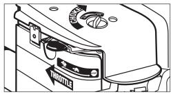
**Step 6** Slide the throttle control to the fast position. Turn the choke control to the "CHOKE" position (only if the engine is cool). After starting, move the choke to "RUN".
