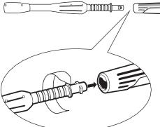
**Step 1** Install the Vario spray wand and set the Vario spray wand to the low pressure setting (-) by turning the wand collar. The wand must be set in the low pressure (-) position to apply detergents.
