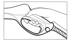
**Step 3** With the engine running, pull trigger to operate unit: Liquid detergent is drawn into the unit and mixed with water. Apply detergent to work area. Do not allow detergent to dry on surface.
