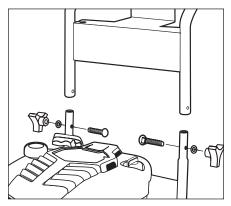
**Step 1** Attach the handle to the frame of the pressure washer. Align holes, insert bolt, and tighten with knob.
