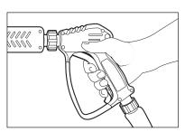
**Step 3** With the engine running, pull trigger to operate unit: Liquid detergent is drawn into the unit and mixed with water. Apply detergent to work area. Do not allow detergent to dry on surface.
