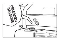
**Step 6** Fill gas tank with unleaded gasoline. Do not use leaded gasoline.
