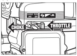
**Step 7** Slide the throttle control to the fast position. Move the choke lever to the "CHOKE" position (only if the engine is cool). After starting, move the choke to "RUN".
