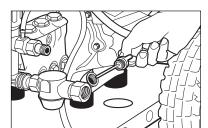
**Step 5** Check oil level. Oil level should be to the oil filler neck. Be sure the machine is level when checking the oil level. (Refer to the engine's operating manual for seasonal grades.)
