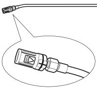
**Step 1** To apply detergents the triple jet nozzle must be set to the "CHEM" position.
