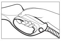
**Step 5** Trigger the gun to eliminate trapped air, wait for a steady flow of water to emerge from the spray nozzle.
