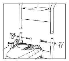
**Step 1** Attach the handle to the frame of the pressure washer. Align holes, insert bolt, add lock washer and tighten with knob.
