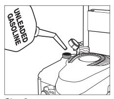
**Step 3** Fill gas tank with unleaded gasoline. Do not use leaded gasoline.
