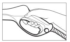
**Step 3** With the engine running, pull trigger to operate unit: Liquid detergent is drawn into the unit and mixed with water. Apply detergent to work area. Do not allow detergent to dry on surface.
