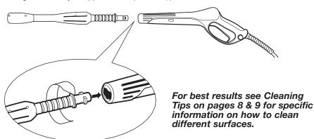
**Step 1** Install the Vario spray wand and set the Vario spray wand to the low pressure setting (-) by turning the wand collar. The wand must be set in the low pressure (-) position to apply detergents.
