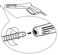
**Step 2** Insert the Vario spray wand into the gun. Push in and turn clockwise to lock spray wand in place.
