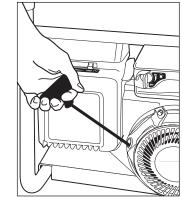
Step 6 Pull the starter handle. If the engine fails to start after 3 pulls squeeze the trigger gun to release pressure, and repeat step 6.
