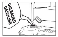
Step 7 Fill gas tank with unleaded gasoline. Do not use leaded gasoline.
