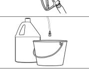
**Step 2** Fill a container with Karcher detergent. Place the filter end of detergent suction tube into the container.
