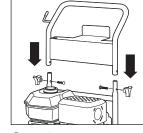
Step 1 Tilt machine backwards slightly (caution: oil may leak if tilted too far). Attach the front guard to the frame. Align holes, insert bolt and tighten with lock nut.
