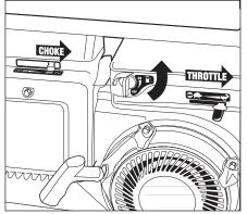
**Step 5** Slide the throttle control to the fast position. Move the choke lever to the "CHOKE" position (only if the engine is cool). After starting, move the choke to "RUN". Turn fuel valve to "ON".
