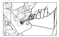
Step 6 Check oil level. Oil level should be to the oil filler neck. Be sure the machine is level when checking the oil level. (Refer to the engine's operating manual for seasonal grades.)
