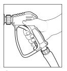
**Step 5** Press trigger to release water pressure.
