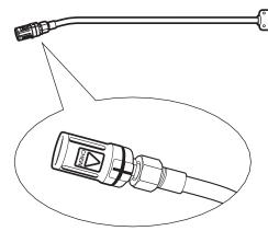
**Step 1** To apply detergents the triple jet nozzle must be set to the "CHEM" position.
