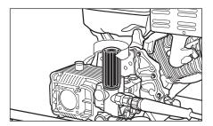
**Step 8** Adjust pressure control to desired setting.
