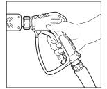
**Step 4** Trigger the gun to eliminate trapped air, wait for a steady flow of water to emerge from the spray nozzle.
