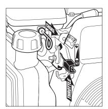
**Step 5** Slide the throttle control to the fast position. Move the choke lever to the "CHOKE" position (only if the engine is cool). After starting, move the choke to "RUN".
