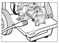
**Step 1** Connect the high pressure hose to the unit's high pressure outlet.
