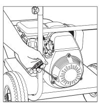
**Step 6** Pull the starter handle. If the engine fails to start after 3 pulls squeeze the trigger gun to release pressure, and repeat step 6.
