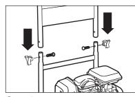
**Step 2** Attach the handle to the frame of the pressure washer. Align holes, insert bolt, and tighten with knob.
