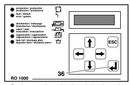
On the control panel, acknowledge the malfunction indication with the RETURN key button (36): the system starts.
