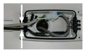
Use the plugs supplied to seal the cable attachment points that are now not required (see illustration on the right).
