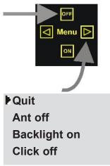
Keep pressing the Up button (OFF) until the cursor is positioned on "Quit" and then press the right arrow button.
