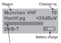
Signal level (RF level) as bar indicator in range 25 to 75 dB $\mu$ V with over/under range indicator.
