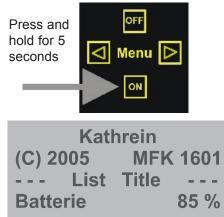
The display first shows the version number and the battery state of charge. The meter automatically switches to the next display readout.
