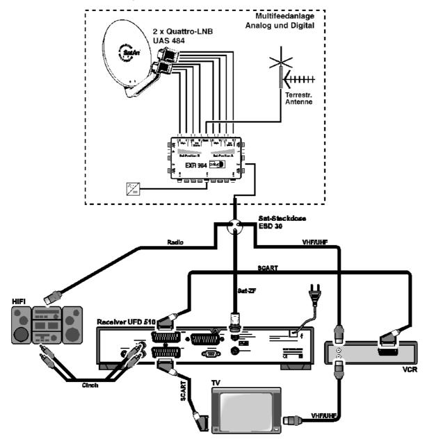
Connection of the UFD 510 digital receiver to a TV set, VCR and a hi-fi system for reception and recording of digital satellite TV- and radio programmes.
