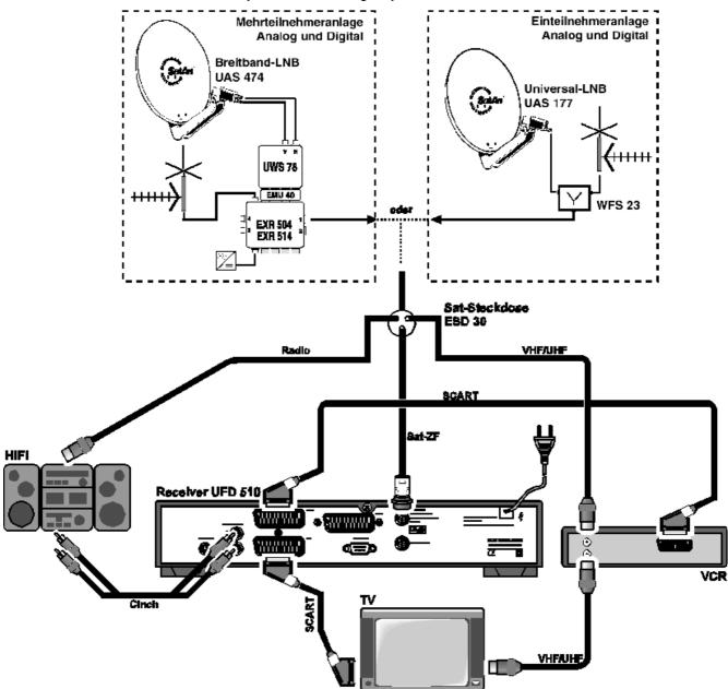
Connection of the UFD 510 digital receiver to a TV set, VCR and a hi-fi system for reception and recording of digital Sat TV- and radio programmes.
