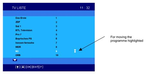
The selected programme is identified by means of a small amber double arrow on the right-hand side of the screen.
