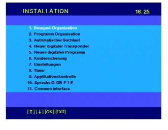
You can select the menu entries using the **V** keys and action them with the **(k**ey. The **(k**ey is used to leave the "Installation" menu.
