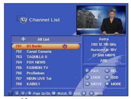
and buttons, you can select the programme, With the which you would like to move. The line with the current running programme will be highlighted with a coloured bar and the programme appears in the upper corner of the screen.
