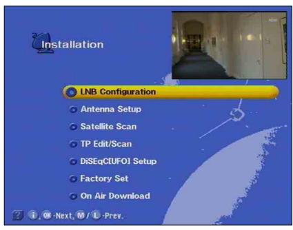
Access the menu item "LNB configuration" via the main menu and the "Installation" - submenu with the and buttons (plus password, if activated). Select this menu item by pressing and then enter or select a new satellite.
