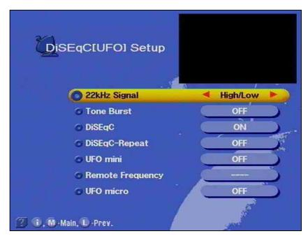
You should only make changes in this menu, when the receiver is connected to another receiving system with different features or if changes have been made to the receiving system.
