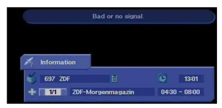
"Bad or no signal" indicates that there is a fault in the receiving system or in the receiver settings. If the transponder is not transmitting any signals, the channel identifier shows a Sat antenna instead of 1.1
