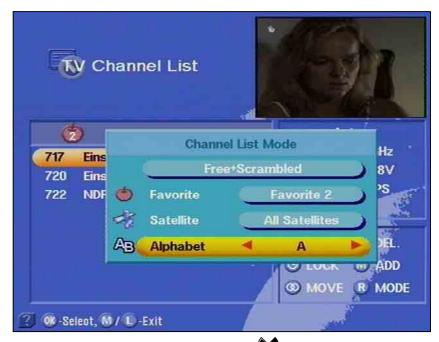
Search for the desired letters using the buttons. The letters can be called up from both directions. Each letter is displayed in the "al-
