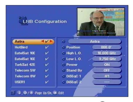
The first submenu is the "LNB configuration". Press to open this menu. Normally, you should not make any changes in this submenu.
