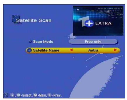
menu 'Satellite search.' With the buttons, move to the menu line. In the first line, select if only free-to-air receivable programmes or free-to-air and scrambled programmes should be searched for using the or button. Set the desired satellite with the or button. Afterwards, the search starts by pressing .
