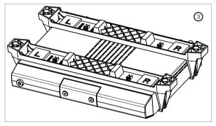
Now take the receiver with the mounting set hooked on to it and place it on the spot where the unit is to be mounted. Screw the supplied wooden screws into the 4 screw holes (see illustration no. 4). If possible, use the wooden screws included in the delivery scope. If this is not possible, other appropriate screws may be used. **Do not under any circumstance use flat-head screws since these can damage the support (see illustration no. 5).**
