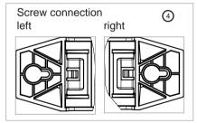
Afterwards, tighten all screws so that the mounting support does not move.
