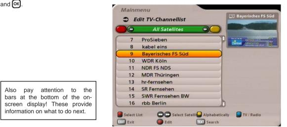
Press the or button to close the information display for editing channels and channel lists. When the menu is called up, the standard setting is for the receiver to show the "All Satellites" channel list with all channels available on the satellites that are being received.
