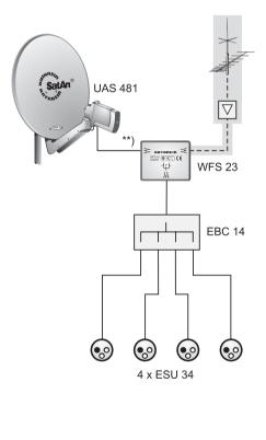
The receiver must be programmed for single-cable commands
