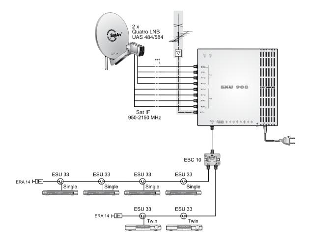
\*) The receiver must be programmed for single-cable commands
