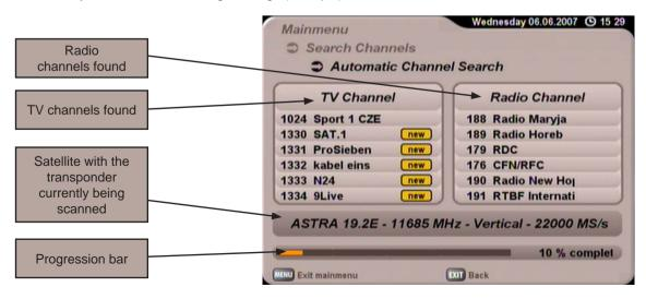
Newly found channels are identified with the designation "new" after the channel name. After completion of the search, you will see the following message (example):
