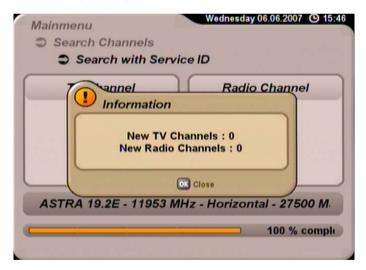
Press the 🔍 button. You will be asked whether you wish to save the changes or not. Selection is performed using the 🔊 buttons and is confirmed using the 🔊 button. If you select "Yes, save changes", the newly found channels will be added to the end of the channel list. Then press the Exit button to exit the menu. The channel list is called up on to the TV screen by pressing the OK button (see also section "On-screen displays" "Channel list TV/Radio").
