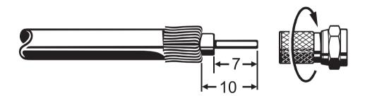
When fitting the connector, make sure that no wires from the braid are touching the inner conductor, so no short circuit can occur.
