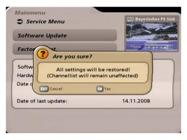
Press the or button to load the factory default settings. The channels and favorites lists remain unchanged.
