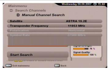
Use the buttons to select the satellite on which the transponder you wish to scan is located. Make sure your reception system is aligned to the selected satellite. You can scan only one transponder at a time. If you wish to scan several transponders on a satellite, you should start an automatic scan
