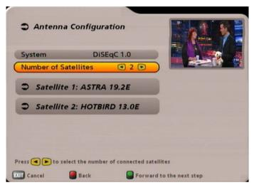
Use the buttons to select the first satellite slot. Press or to access the menu for the satellite settings. The following display appears (example):
