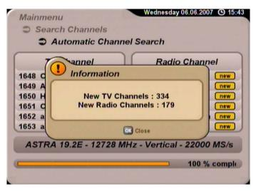
Press the OK button. You will be asked whether you wish to save the changes or not. Selection is performed using the AV buttons and is confirmed using the OK button. If you select "Yes, save changes", the newly found channels will be added to the end of the channel list. Then press the EXT button to exit the menu. The channel list is called up on to the TV screen by pressing the OK button (see also section "On-screen displays" "Channel list TV/Radio").
