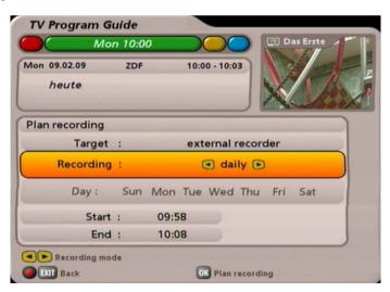
When all settings have been made, press the object button to save the recording settings. You can view the recording in the Timer List view of the EPG (see item "Plan recording").
