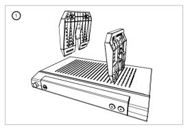
Remove the wood screws supplied from their transport attachment on the underside of the respective mounting piece (2 pieces).
