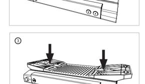
Now press the mounting pieces firmly against the receiver casing at the points shown arrowed in Fig. 3), until the catch audibly snaps home in the receiver casing.
