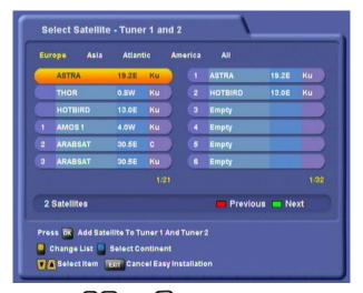
Press the A and k buttons here to select the satellites you want tuners 1 and 2 to receive signals
