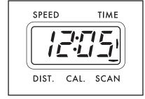
scan mode is selected, and a flashing mode indicator will show which mode is currently displayed. Note: If a different mode is selected, you can select the scan mode again by repeatedly pressing the mode button. Speed, time, distance or calorie mode—To select one of these modes for continuous display, press the mode button repeatedly.
