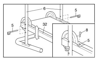
the Frame, align the holes in the Frame with one of the three sets of holes in the Handrail (6), and reinsert the Long Pins. **Make sure both Long Pins are at the same level.** Refer to the inset drawing. Insert a Cotter Pin (8) into the hole in each Long Pin. **Make sure that the Long Pins are fully inserted into the holes.**
