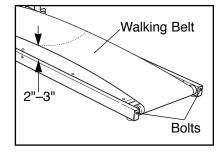
Using the allen wrench, turn both rear roller adjustment bolts counterclockwise 1/4 of a turn. When the tension of the walking belt is correct, you should be able to lift each side of the walking belt 2 to 3 inches. Walk on the treadmill for a few minutes. Repeat until the walking belt is properly tightened. Be careful to keep the walking belt centered.
