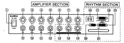
① POWER switch : turns the unit's power on or off.
