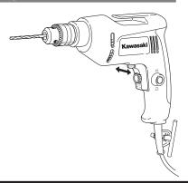
**CAUTION** Do not change the direction of a moving bit. Make sure the bit comes to a complete standstill before moving switch. Changing direction while the bit is moving can cause damage to the drill.
