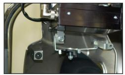
Route the harness from the CB module behind the left engine guard and into the left side of the fairing. Find the matching multi-pin connector at the left side of the radio and connect to the CB module harness. Press the connectors together firmly to engage the waterproof seals. Secure the cables as needed with provided cable ties.
