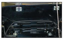
Cut the antenna base drilling template out of the instruction sheet. Carefully fold it at the score lines and tape to the inside right rear corner of the trunk as shown.
