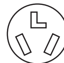
3-wire receptacle (10-30R)
