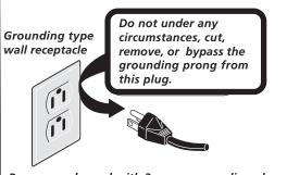
Power supply cord with 3-prong grounding plug
