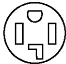
4-wire receptacle (14-30R)
