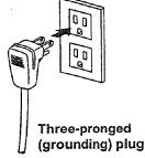
This appliance must be grounded. In the event of an electrical short circuit, grounding reduces the risk of electric shock by providing an escape wire for the electric current. This appliance is equipped with a cord having a grounding wire with a grounding plug. The plug must be plugged into an outlet that is properly installed and grounded.
