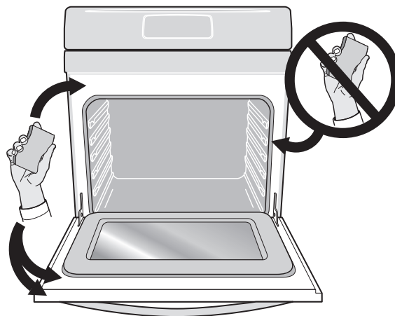
Figure 18: Oven door area to clean and not clean (gasket).
