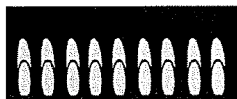
(C) Soft blue flames—Normal for natural gas
