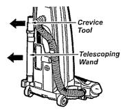
Remove the telescoping wand from its storage position.
