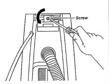
Remove the screw located just below the top edge of the back of the vacuum.
