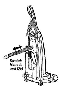
Plug in the vacuum and turn it on. Stretch the hose to maximum length and then allow the hose to return to its storage length.
