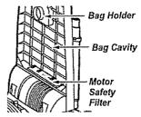
Check the bag holder and the motor safety filter. If either is blocked, check TROUBLE-SHOOTING.
