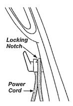
Wrap the power cord around the upper and lower cord hooks and lock the power cord plug onto the power cord.
