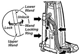
Unlock the wand by turning the wand locking ring to the **UNLOCK** position.
