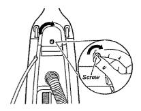
Begin to tighten the screw with your fingers It may be necessary to adjust the handle slightly.
