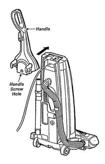
Insert the screw so it passes through the handle into the vacuum.
