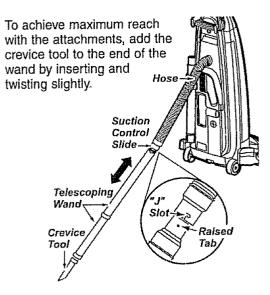
When using the dusting brush or the combination brush, they may be attached directly to the wand or placed on the end of the crevice tool.
