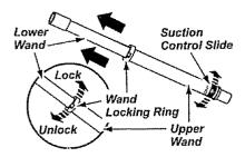
Align the tabs on the extension wand with the "J" slots in the hose. Push the wand into the hose and twist to the right to lock.
