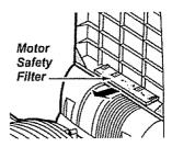
2. If the filter, located in the bottom of the bag cavity, is dirty, remove it by pulling forward out from under the ribs.
