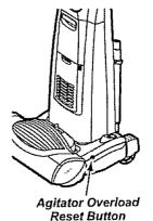
The agitator has built-in protection against motor damage should the agitator jam. If the agitator slows down or stops, the agitator overload protector shuts off the agitator. The suction motor will continue to run.
