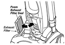
The foam seal of the filter should be placed against the vacuum cleaner body
