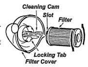
Clean primary filter by gently tapping over a trash container. Tap on several sides to ensure best cleaning. Rinse with water only as needed, do not use any detergent or soap. Allow the filter to dry for 24 hours before putting it back into the vacuum.
