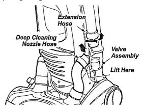
Visually inspect the hose and the base area into which the hose is connected.
