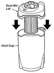
Replace dust bin lid assembly by placing back on dust cup as shown.
