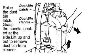
Remove any clogs that might be located in the dust bin port or the filter screen.
