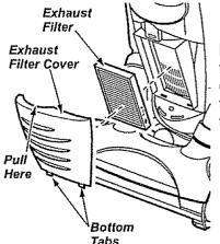
Remove the exhaust filter cartridge.
