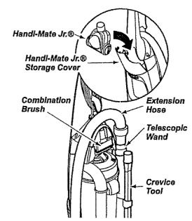
Remove crevice tool from the wand by twisting. Place in wand holder.
