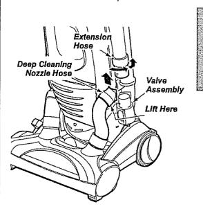
To clean the sensor, remove deep cleaning nozzle hose at valve assembly by lifting hose straight up. Remove extension hose from the valve assembly by grasping hose collar, twisting, and pulling straight off.
