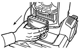
Return exhaust filter to cleaner. Replace exhaust filter cover by inserting the tab on the cover into the slot on the cleaner. Pivot toward cleaner until cover snaps into place.
