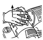
4. Insert flat blade of screwdriver into slot at top of the lens. Lift the lens cover to remove.
