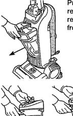
Press dirt container release button and remove dirt container from cleaner.
