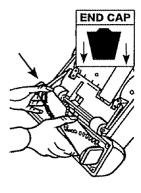
With new belt in place, pull and slide brushroll into nozzle making sure that the brushroll end caps are in the correct orientation (see diagram for end cap orientation). Rotate brushroll manually to make sure belt is properly aligned.
