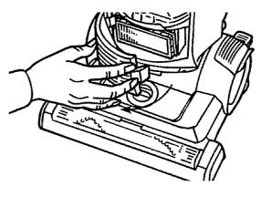
Remove exhaust filter from cleaner. Tap filter on inside of garbage can to remove excess dust and dirt from filter.
