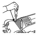
**3.** Remove the two (2) screws from the lens cover.
