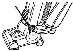
Rotate the handle and adjust it to the desired position for (A) storing the upright, (B) operating the cleaner, and (C) to clean under furniture. **NOTE:** Rotating brush could cause area rug fringe to become tangled within cleaner. Use caution when vacuuming any rugs with fringe.
