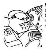
**5.** Pull bulb out of socket. Do NOT twist. Gently push replacement bulb into socket to replace.
