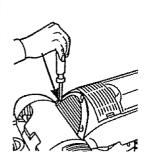
6. Snap lens cover back into place and secure the headlight lens by replacing the two screws.
