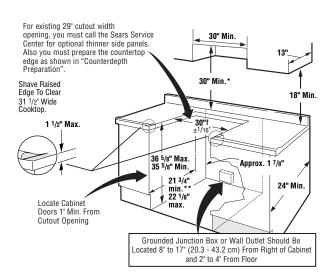
Do not pinch the power supply cord between the range and the wall. Do not seal the range to the side cabinets.
