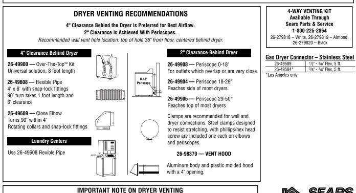
Do not use non-metal flexible duct. When installing the venting system, do not exceed the specified length for the vent duct. Venting systems which are longer than specified will accumulate lint, increase drying time and energy use and shorten the life of the dryer.
