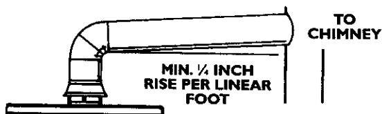
VENT PIPE INSTALLATION
