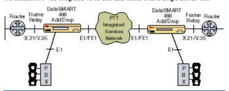
With in-band management and local Ethernet connectivity, the DataSMART 486 and 488 can be managed easily from a remote or local site. The management system can be located anywhere on the business network.
