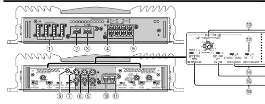
This is a 4 channel amplifier including 2 stereo amplifiers in a body. One amplifier is referred to as amplifier A and the other is amplifier B. This unit is compatible with a large variety of systems by combining the switches and functions described in the following.
