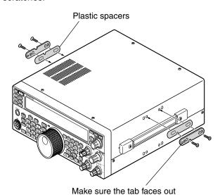
Once the bracket is installed onto the vehicle, prepare the transceiver by loosely screwing in the rear screws. Hook those screws onto the rear guide rail of the mounting bracket then adjust the transceiver to your desired angle before tightening the screws. Insert and tighten the front screws to secure the transceiver in place.
