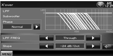
**[Phase]** Sets the phase of subwoofer output. The phase is reversed 180 degrees when set to "Reverse".
