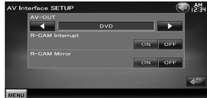
**[AV-OUT]** Selects an AV source to be output at the AV OUTPUT port. (☑ "AV-IN1")
