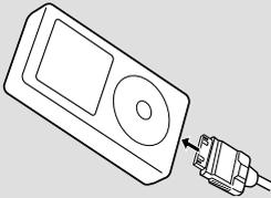
To disconnect the iPod, stop the playback by touching the [▶||] button on the source control screen, and then disconnect the iPod. See <Source Control Screen> (page 29).
