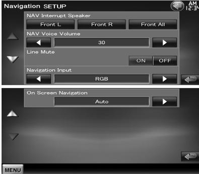
**[NAV Interrupt Speaker]** Selects speakers used for voice guidance of the navigation system.
