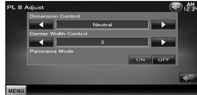
**[Dimension Control]** Sets the surround position by adjusting the front and rear volume balance.
