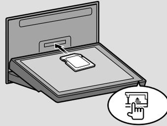
Press the [▲] button for more than 1 second to open the front panel.
