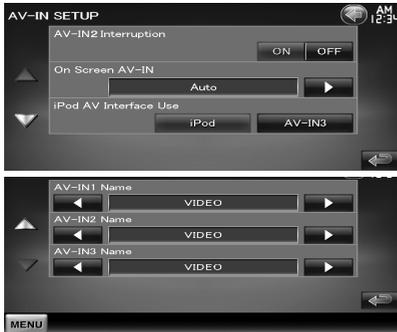
**[AV-IN2 Interruption]** Sets an image display of the system that is connected via the AV INPUT2 port. (☑ "OFF")
