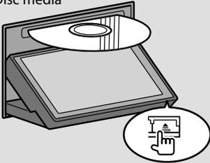
Press the [▲] button to open/close the front panel.
