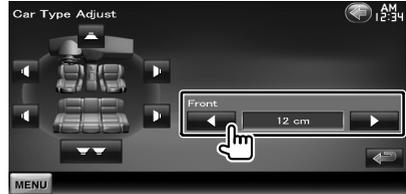
Make fine adjustment of the delay time of the speaker output specified at <Setup the Car Type> to have a more suitable environment for your vehicle.
