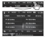
The preset list and the station name for FM Radio Data System (when PS signal is coming in) are displayed.
