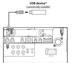
\* Use CA-U1EX for extending the cable if necessary. (Max 500 mA, 5V)
