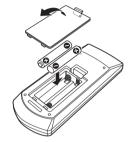
If the Remote Controller operates only over shorter distances or does not operate at all, it is possible that the batteries are depleted. In such instances, replace both batteries with new ones.
